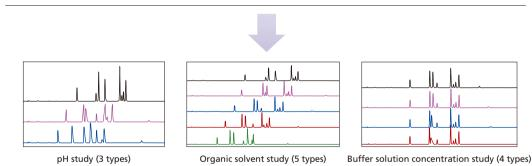
12 types of mobile phases were prepared and analyzed automatically by the system.
