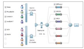
Simply select the checkboxes for mobile phases and columns to use, and a method will be created automatically.
