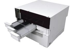
The Nexera MP system is able to access samples via the quickest path by moving the needle in both X and Y directions simultaneously. This achieves higher injection speeds than ever before, with shortest injection time being about 7 seconds.
