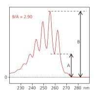
In addition, the new signal treatment technology realizes excellent spectrum linearity across a wide area from low to high concentration. The SPD-M30A supports analyses, such as purity analysis, that require a wide dynamic range.
