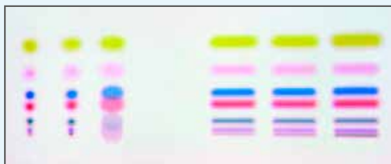
Separation of a test dye mixture on HPTLC silica gel; always CAMAG Test Dye III (from left) diluted 1:1 with hexane, toluene, or methanol respectively, contact spotting 2 \mu L each, bandwise spray-on application of 6 \mu L as 10 mm bands with Linomat 5; development with toluene. It can be seen that the result for contact spotting is strongly dependent on the solvent of the sample, whereas for bandwise spray-on application this is not the case. Furthermore, the separation is significantly improved.
